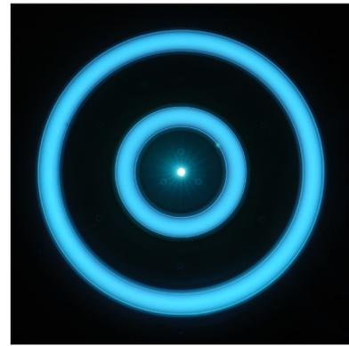
**Figure 22.** Front view of the 10 kW class X2 two-channel nested Hall thruster with its centered-mounted cathode firing with xenon at full power in dual channel configuration. Image courtesy of Ray Liang, reproduced with permission.
