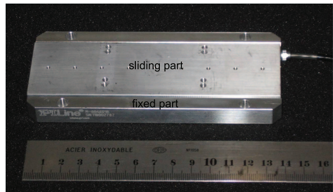
FIG. 1. Picture of the ultrasonic piezo PILine ® Linear Motor Stage M664K018. The sliding and the fixed part of the linear drive are marked.
