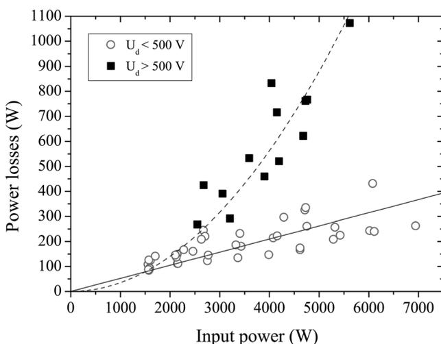
FIG. 4. Power losses on walls against input electrical power. Data is divided into two groups:  $U_d < 500$  V and  $U_d > 500$  V. Solid line is a linear fit. The dashed line is a power law fit ( $P^{1.6}$ ) through the high voltage range.
