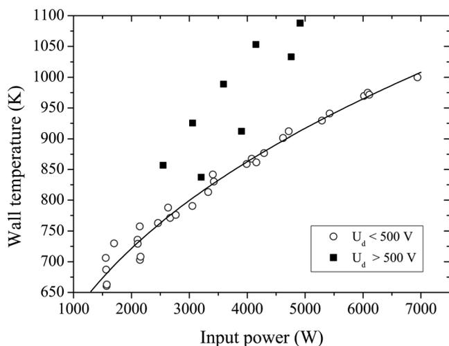
FIG. 1. Equilibrium wall temperature against input power. Datapoints are split into two groups:  $U_d < 500$  V and  $U_d > 500$  V. The line corresponds to a curve fitting with the power law  $T_{\text{wall}} \propto P^{0.38}$ .
