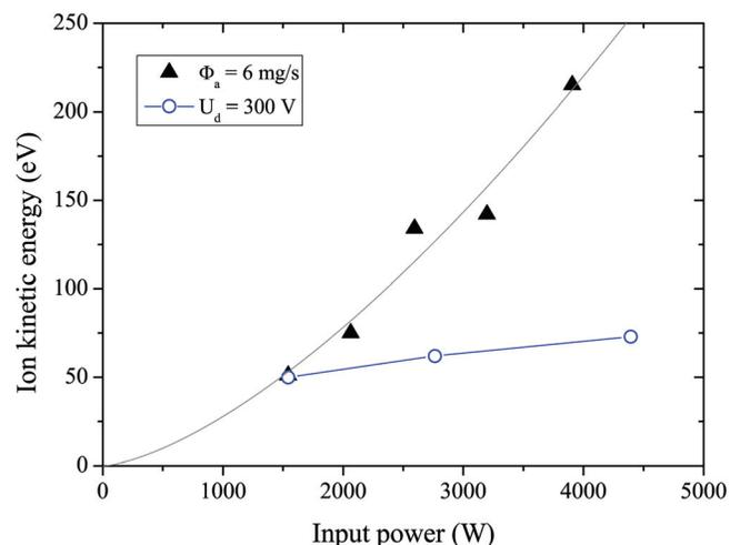
FIG. 5. (Color online) Xe<sup>+</sup> ion axial kinetic energy at the channel exhaust against applied power: mass flow rate series at 300 V (circle), voltage series at 6 mg/s (triangle). The line is a power function fit ( $P^{1.5}$ ) to voltage series points.
