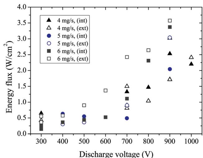
FIG. 2. (Color online) Power per unit area  $q_p$  delivered by the plasma onto the channel dielectric walls against the discharge voltage: internal wall (full symbol) and external wall (open symbol). The xenon mass flow rate is varied from 4 to 6 mg/s.
