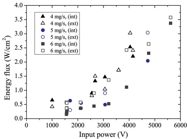
FIG. 3. (Color online) Power per unit area  $q_p$  delivered by the plasma onto the channel dielectric walls as a function of the input electrical power for three values of the mass flow rate: internal wall (full symbol) and external wall (open symbol).
