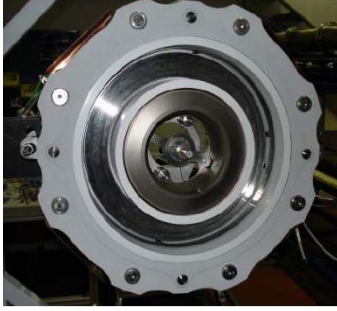
Figure 3.11: Picture of the 20 kW-class PPS-20k ML Hall thruster with the cathode mounted in the center of the thruster.
